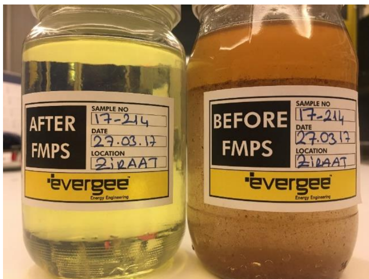
Right-before fuel polishing, Left- after fuel polishing
