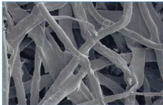
Unused paper element at x270 magnification
